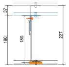
180 Bracket ADJUSTMENT= +/- 37mm Clad Zone= 190mm to 227mm
