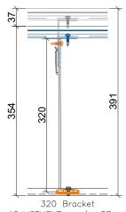
ADJUSTMENT= +/- 37mm Clad Zone= 354mm to 391mm
