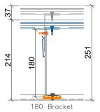
ADJUSTMENT= +/- 37mm Clad Zone= 214mm to 251mm
