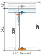
ADJUSTMENT= +/- 37mm Clad Zone= 254mm to 291mm
