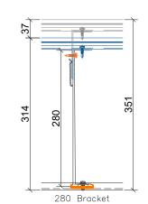
ADJUSTMENT= +/- 37mm Clad Zone= 314mm to 351mm
