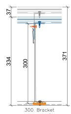
ADJUSTMENT= +/- 37mm Clad Zone= 334mm to 371mm
