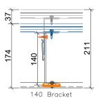
ADJUSTMENT= +/- 37mm Clad Zone= 174mm to 211mm
