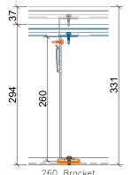
260 Bracket ADJUSTMENT= +/- 37mm Clad Zone= 294mm to 331mm
