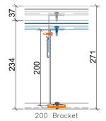
ADJUSTMENT= +/- 37mm Clad Zone= 234mm to 271mm
