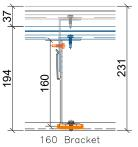
ADJUSTMENT= +/- 37mm Clad Zone= 194mm to 231mm
