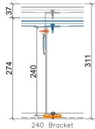
ADJUSTMENT= +/- 37mm Clad Zone= 274mm to 311mm
